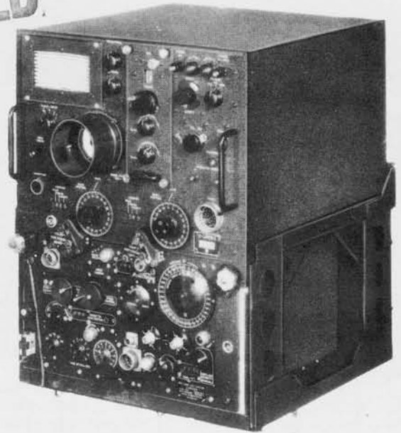
Indicator ID-17/APN-3 On Mounting MT-216/APN-3
