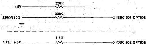
Ports 1, 4, and 7 may use any of the drivers or terminators shown above for unidirectional (input or output) port configurations. Either terminator and the following bidirectional drivers and terminators may be used for ports 1, 4, and 7 when these ports are used as bidirectional ports.
